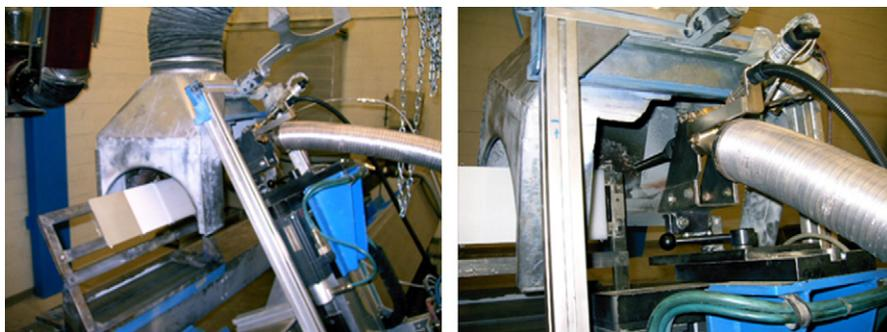
Fig. 3. Kinetic 3000 Cold Spray System operated at Freiburger NE-Metall GmbH & Co Produktion KG, Freiberg, Germany (left) and close-up view of the spray nozzle (right). Coated polymer samples are shown on the rack in the left image.
